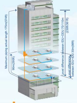
The solution supports an incredible piping length of 1,000m(3280ft) and level difference of 110m(361ft), making it perfect for large projects.
