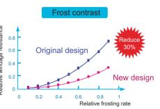
Hydrophilic fins + inner-threaded pipes
