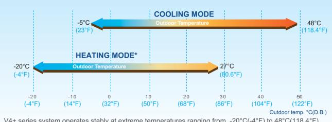
The V4+ series system operates stably at extreme temperatures ranging from -20°C(-4°F) to 48°C(118.4°F). \*V4 Plus C system is without HEATING MODE.
