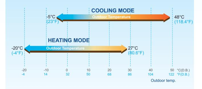
The V4+ S series system operates stably at extreme temperatures ranging from minus 20°C to 48°C. (-4°F to 118.4°F)
