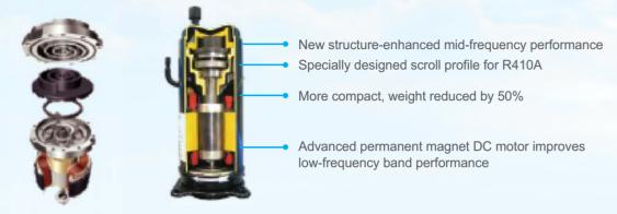
Powerful magnets provide high torque and efficiency and achieve 70% reduction in volume.
