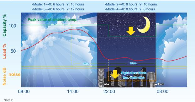
This function can be activated by setting at site. Temperature(load) curve shown in the graph is just an example.
